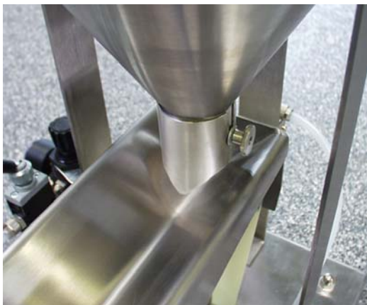
Dosing port at the silo outlet
